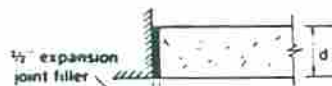
DETAIL F Use only at buildings or objects abutting the paved area.
