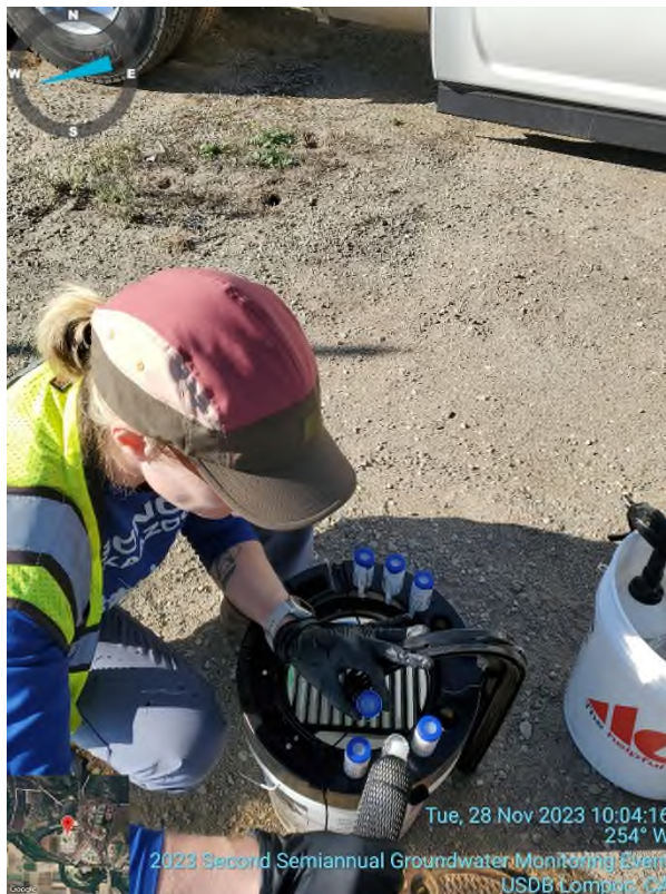
Photo #2: Collecting water samples from passive diffusion bags (PDBs).
