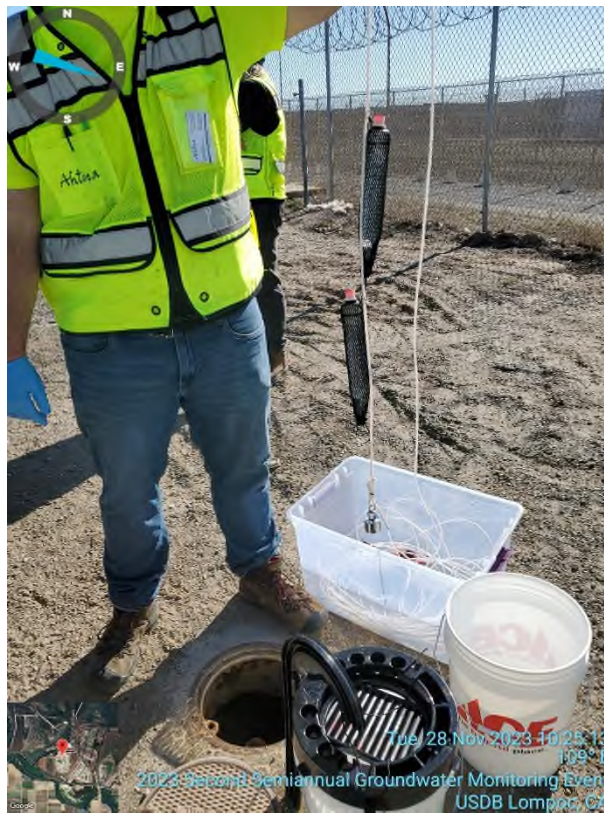
Photo #3: Primary and Duplicate PDBs set at WR-MW-08A.
