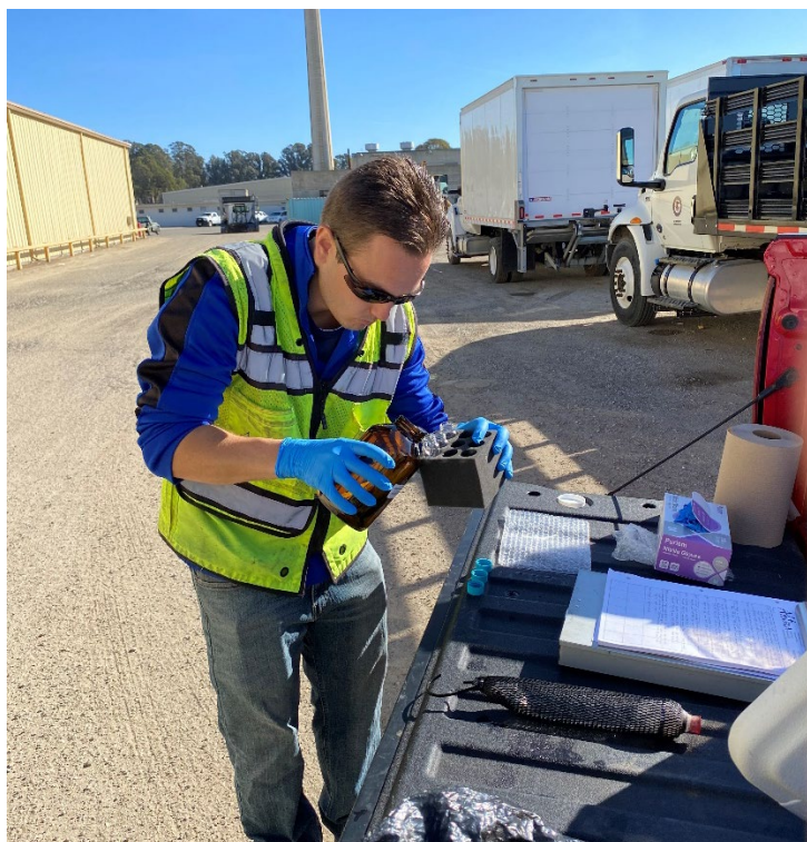
Photo 02: Collecting field blank sample using laboratory-provided DI water (facing east).
