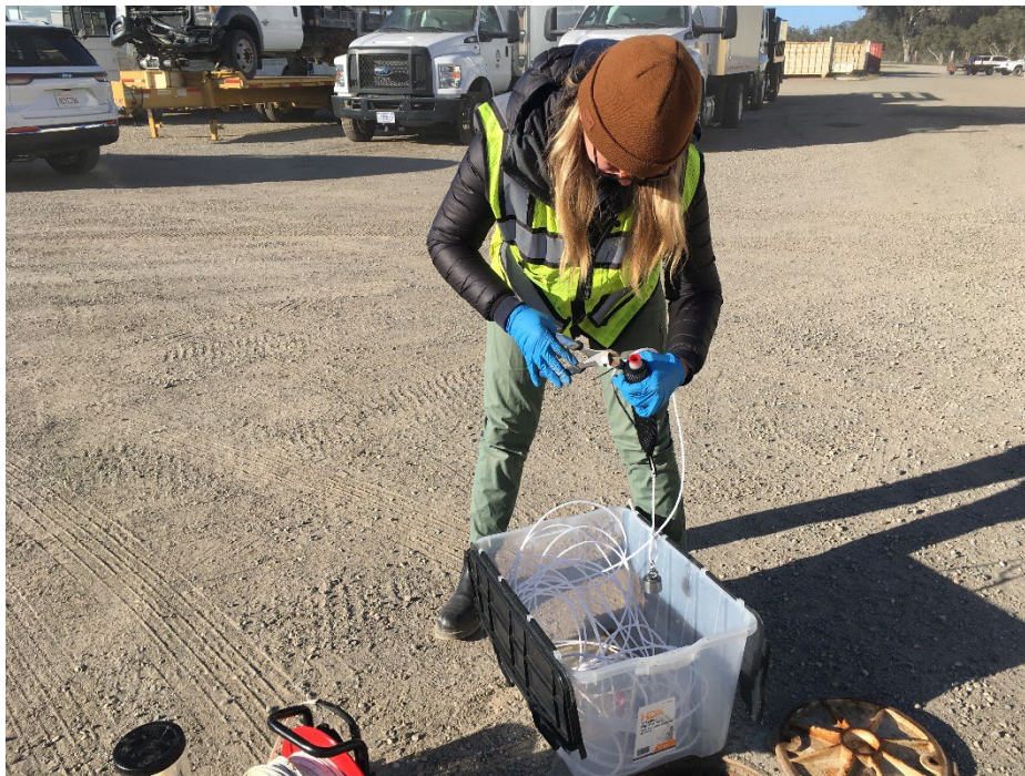
Photo 01: Retrieving PDB from well WR-MW-01 (facing west).
