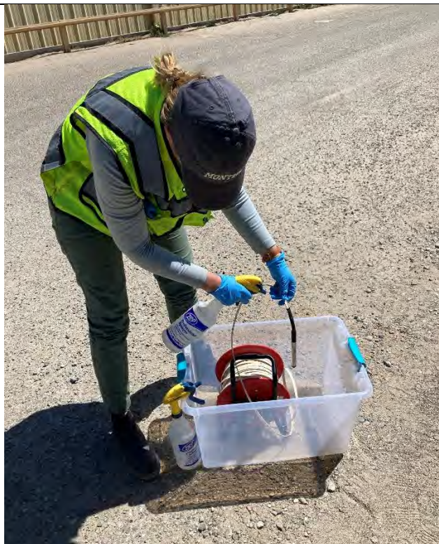
Description: Decontaminating water level sounder before use at WR-MW-12A, facing north
