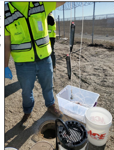
Removing PDBs from well WR-MW-08A for sample collection
