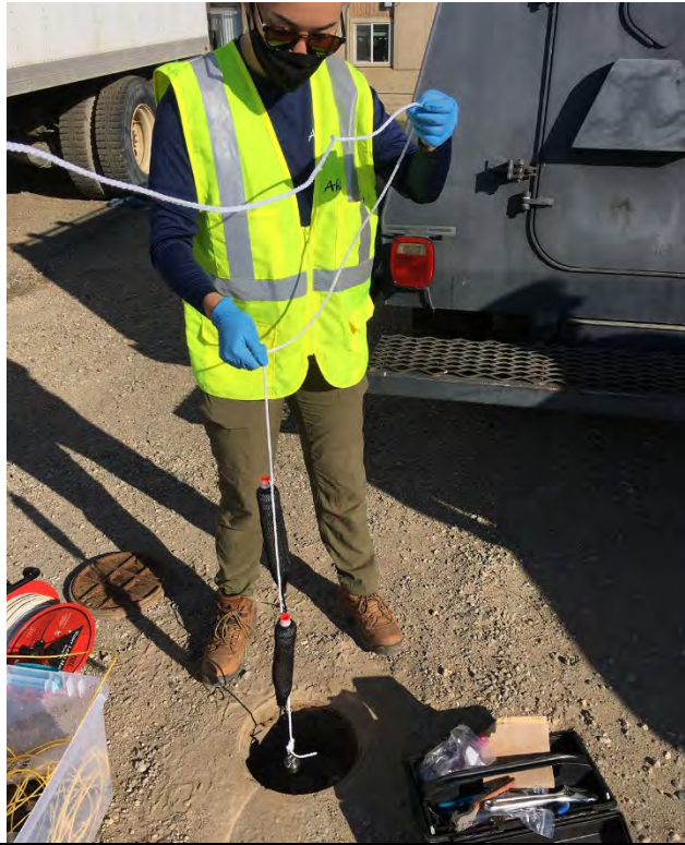
Description: Setting Field Duplicate passive diffusion bags (PDB) at WR-MW-02, facing east.
