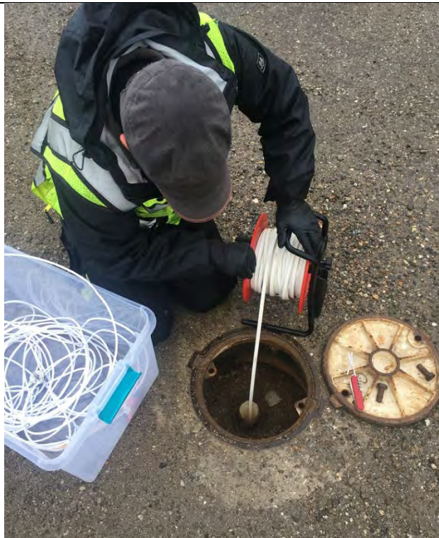
Description: Collecting a depth to water measurement using a sounder at WR-MW-05A, facing north
