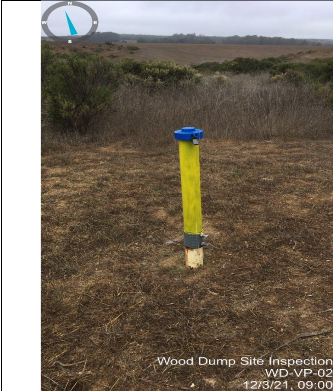
Photo 17: Vapor probe, WD-VP-02, facing north.
