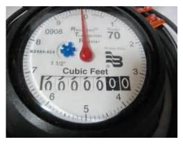
If the needle has moved or the numbers have changed, you have a leak (probably a slow one. If you have a larger leak, you will see the needle moving right away.) One rotation of the red dial is about 7.5 gallons.
