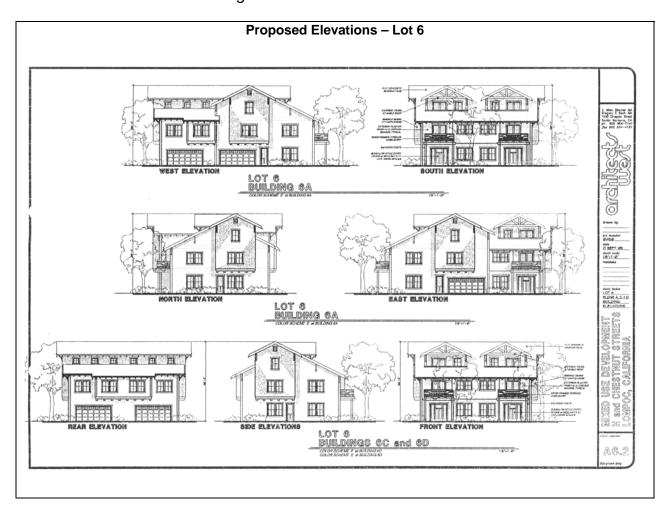
The proposed architecture for buildings on Lot 6 present a more residential type appearance more appropriate to the G Street area. The buildings are three story with bungalow style entry doors, shingle siding on cantilevers, with exterior plaster finish and wood framed terrace over the entry.
