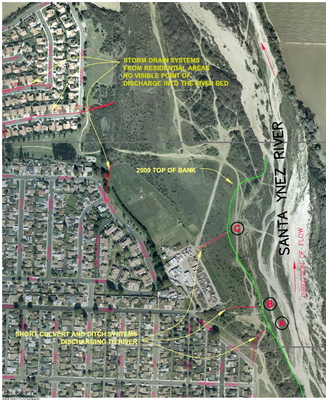
Figure G - Storm Water Outfalls
