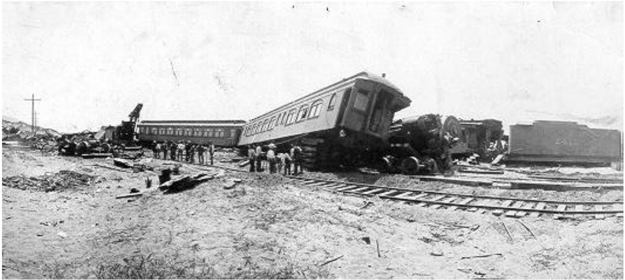
Shriner's train wreck on May 11, 1907. At 55 mph the drive wheels jumped off the tracks and snapped off. The cowcatcher buried in the ground and crushed the boiler. The Engineer was ejected from the train and survived. 32 People were killed.
