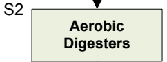
S1 - DAFT: sludge is pumped to the DAFT by the waste mix liquor (WML) pumps where final conditioning is done before treatment in the aerobic digesters.
