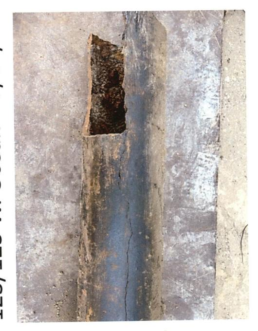
Section removed in two pieces after bottom of pipe ruptured
